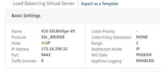
5. Add a **Binding** to the load balancing server group, binding the ICG-SSLBridge Service you created in step 2.
