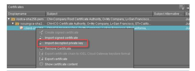
(i) If the private key is protected with a passphrase, you need to decrypt it using the OpenSSL command line tool: openssl rsa -in encrypted.key -out decrypted.key
