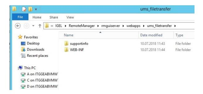
5. After file synchronization, the file is present on the file system of server B (v-j-mv-umstest3), but the file object is not visible yet on the UMS console connected to server B.
